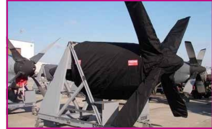
Protective Packaging for Aircraft Parts
